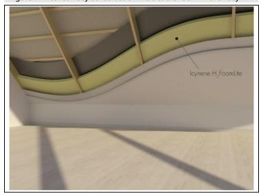
Figure 1 Pitched roof construction: habitable room in the roof
