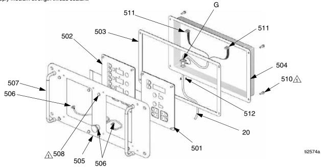
Detail of Membrane Switches and Display Boards
