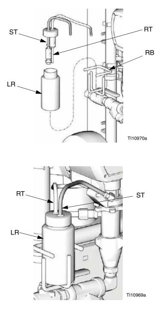
FIG. 13. Pump Lubrication System
