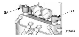
6. Disconnect gun air line and remove gun fluid manifold.
