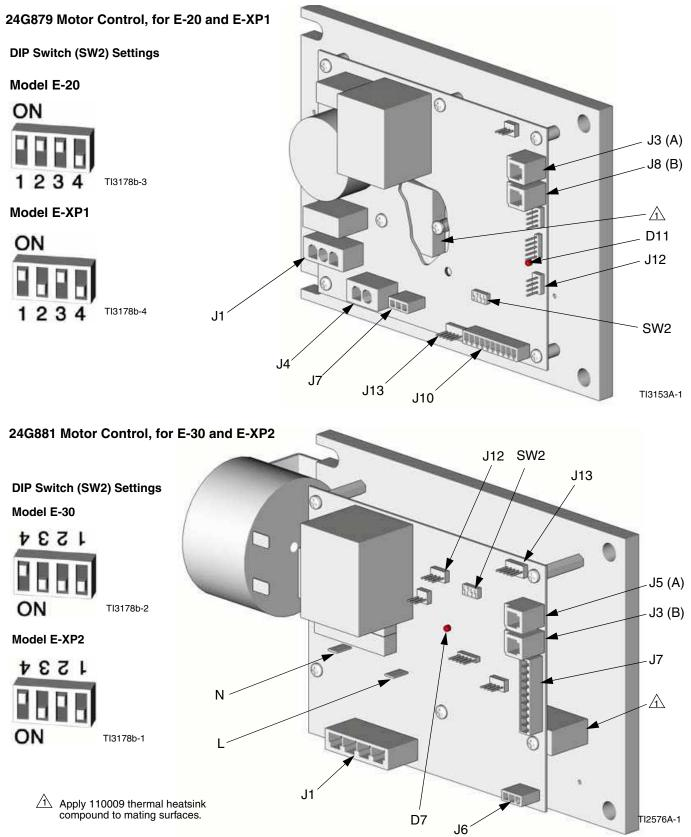
FIG. 2. Motor Control Board
