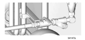
Turn both PRESSURE RELIEF/SPRAY valves (SA, 6. SB) to PRESSURE RELIEF. Route fluid to waste containers or supply tanks. Ensure gauges drop to 0.
