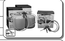
Handi-Foam® E84 Class 1 Spray Foam is a low pressure foam system that utilizes a non-flammable blowing agent. Handi-Foam E84 Class 1 Spray Foam has been specifically formulated for flame retardancy and conforms to the requirements of ASTM E84 as a "Class 1(A)" system (flame spread of 25 or less, smoke development of 450 or less). The foam helps to lower heating and cooling costs by drastically reducing energy consumption.
