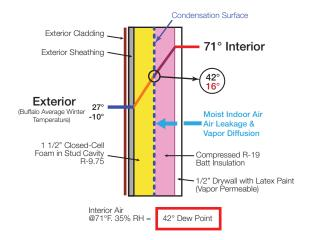
This wall section has an acceptable thickness of closed-cell spray foam to be a Class II vapor retarder. Condensation is less likely during average winter temperatures, but an extremely cold period can create issues, even with a total R-value (28.75) much greater than the required R-20. This wall assembly will allow the wall to dry towards the interior, when temperatures rise, but does not remove the risk of moisture forming to begin with.
