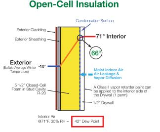
This wall section is properly designed using open-cell spray foam insulation and a Class II vapor retarder (required in Climate Zones 5, 6, 7, 8 and Marine 4), applied to the interior side of the wall assembly. This wall assembly meets all prescriptive building code requirements for R-value and vapor retardance, and removes most risk for condensation forming.
