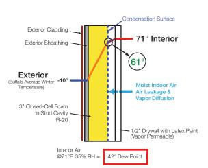
This wall section is properly designed using closed-cell spray foam. The applied thickness meets the minimum required R-value and is adequate to achieve a Class II vapor retarder rating. This wall section effectively places the vapor retarder layer on the interior side of the wall, and removes most risk for condensation forming.
