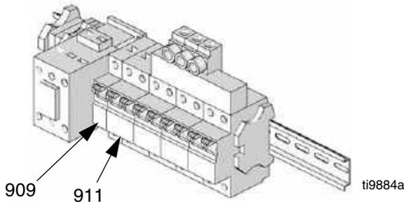
**FIG. 10: Circuit Breaker Module**
