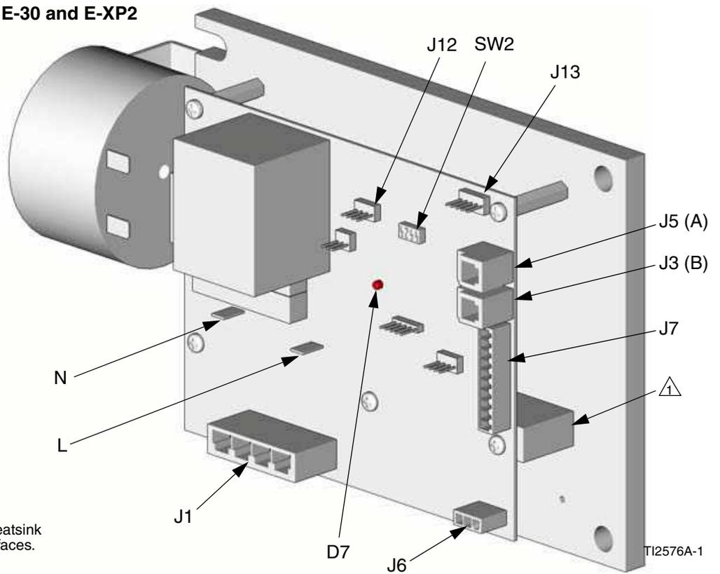
⚠ Apply 110009 thermal heatsink compound to mating surfaces.
