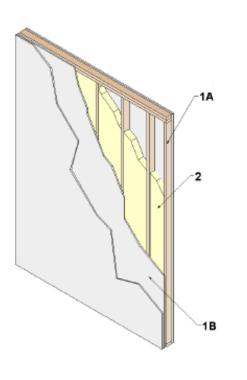
1A. WOOD STUDS: Install nominal 2-inch-by-4-inch Number 2 Southern Yellow Pine wood studs spaced maximum 16 inches on center.
